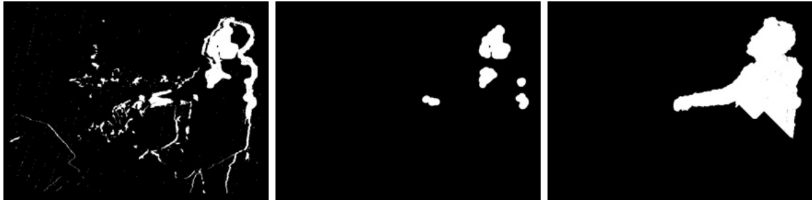
Figure 3.3: Illustration of the stages of mask generation. From left to right: post-thresholding, post-opening and post-flood-fill (final mask).
